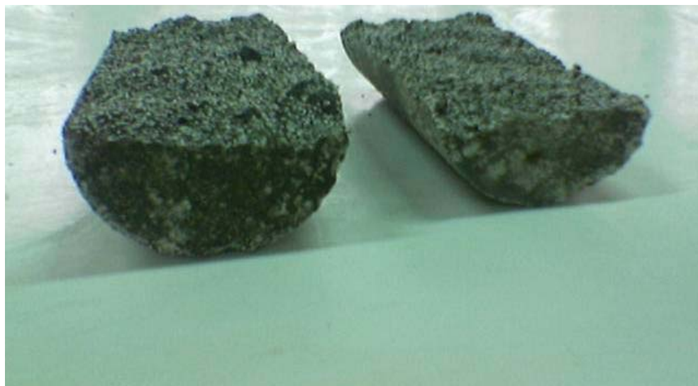
Figure 21. The failure mode in EPS glasscrete.
