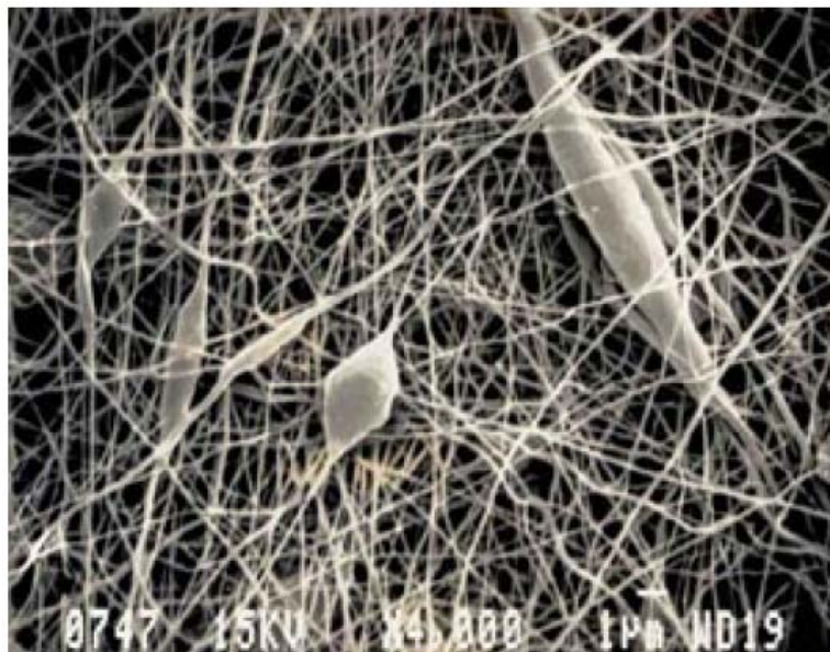
Figure 9. SEM images of nonuniform electrospun nanofibers.
